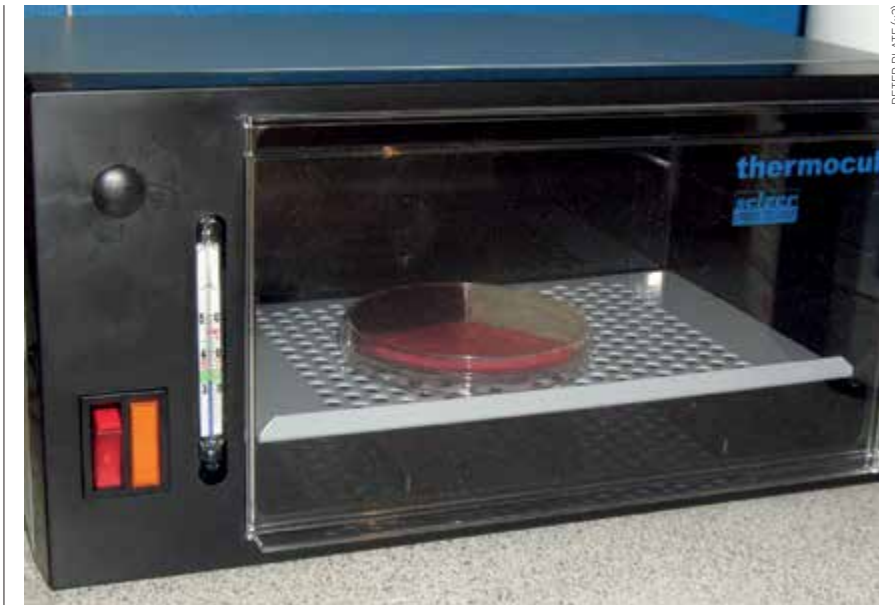
Culture plates are incubated for 18-24 hours on the farm. Incubators range from $70 for a plastic foam egg incubator to $300+ for a lab incubator
